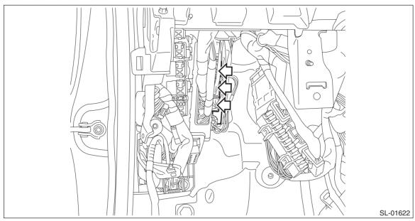
(2) Release the claws, and pull out the keyless access CM from the bracket.
